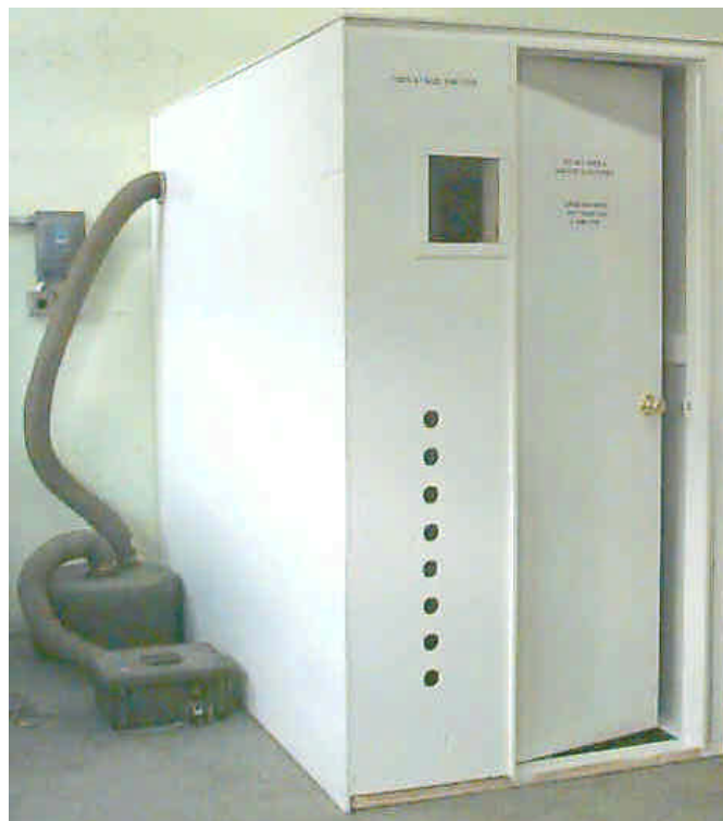
Figure J-5. Fabricated Airlock with Filter-Blower Unit
